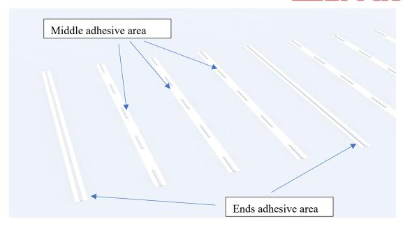
■ Paste the rail along the gluing path and lightly compress. Ensure the bead height is not less than 3mm
